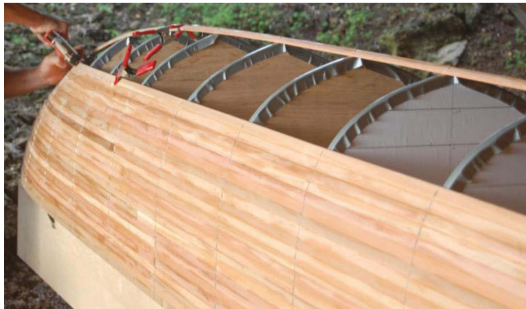
Figure 17: Strip-planking Construction Source: John Ashley
