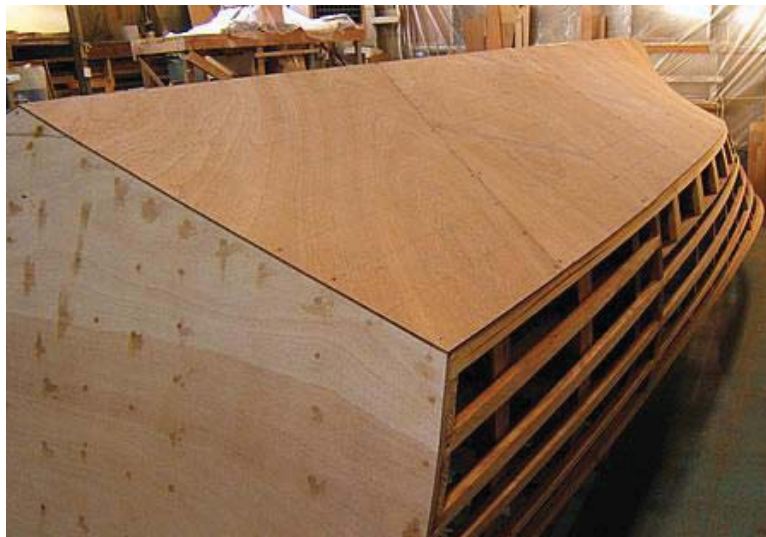
Figure 15: Cold-molded Construction Source: Nexus Marine
